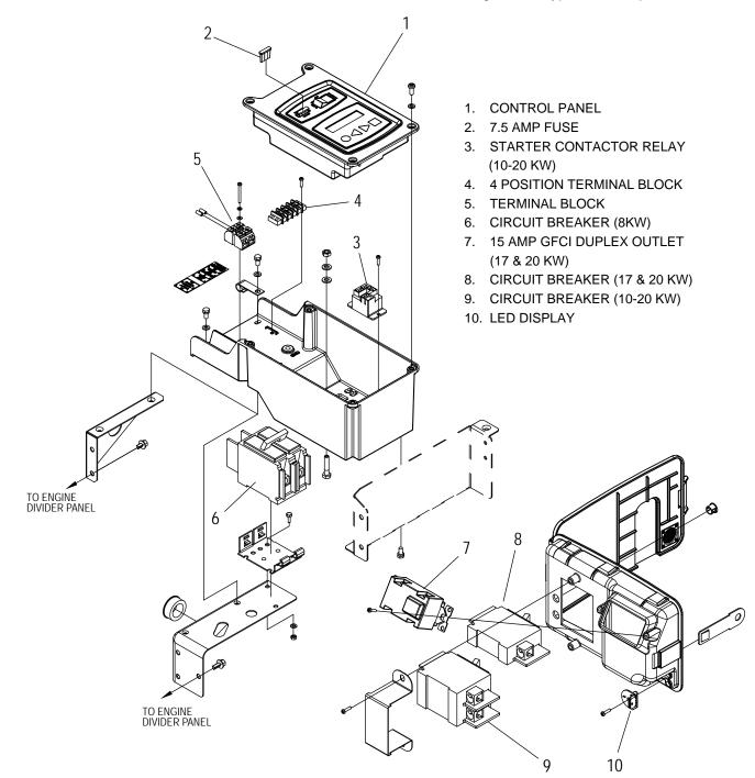
Figure 3. Control Panel Component Identification
